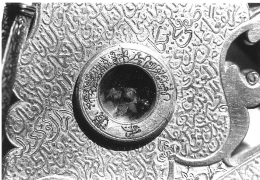
Fig. 2. A compass about 15 mm in diameter on the throne of an astrolabe made by Muhammad Mahdī ca. 1050/1650. Photo by D.A. King, courtesy of the National Maritime Museum, Greenwich.
